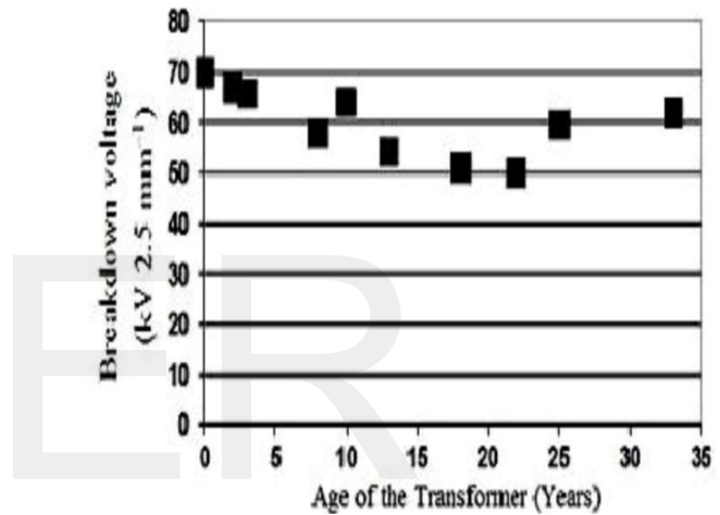
Figure 13 Breakdown voltage of the oil specimens from transformers of different ages [8]
